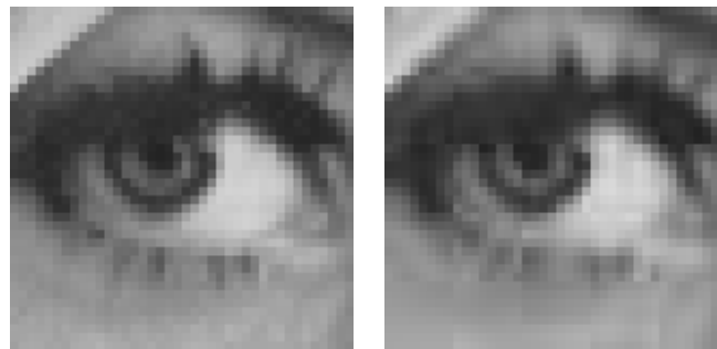
Figure 5. Original grayscale Lena image zoomed in to 400% (left) and the output image from DCT standard JPEG quantization (right).
