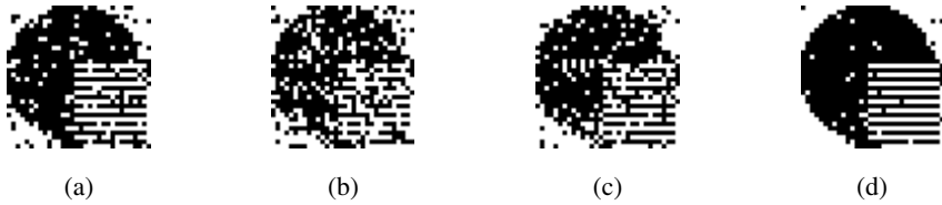
Fig. 7. The extracted watermark image after from (a) JPEG image compression, (b) Gaussian white noise 0.01, (c) Salt and pepper 0.02 and (d) 3 \times 3 Gaussian low pass filter
