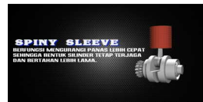
Gambar 56. Pengertian spiny sleeve
